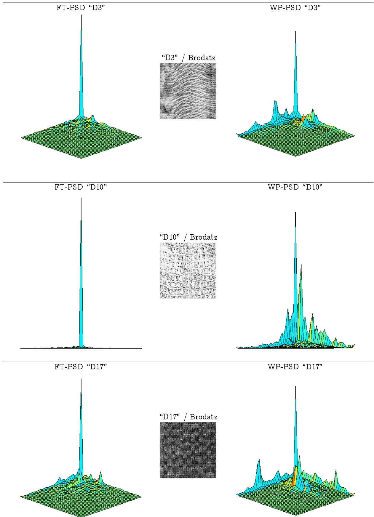
Fig. 1. Texture images and their spectra  $\hat{\gamma}$  computed by using Fourier and wavelet packets. Abscissa of the spectra images consist of a regular grid over  $[0, \pi/2] \times [0, \pi/2]$ .
